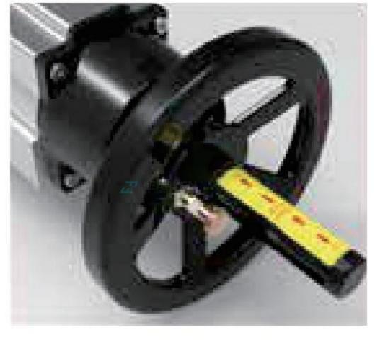
Quick and Safe manual switching The manual lock is a spring stop pin. Pull out the pin and rotate 45° to unlock and start manual operation. Rotate the handwheel to pneumatic mode position, the stop pin will work andhandwheel operation stopped.
