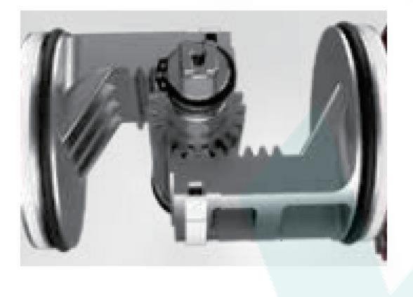
Output Shaft: The one-piece high precision output shaft is made by alloy steel and chrome coated. It complies with NAMUR, ISO 5211 and DIN 3337 at the same time. Customized dimensions and materials are available.
